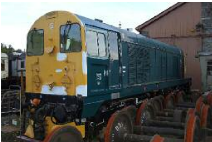
Cab repainting and touching up underway.
