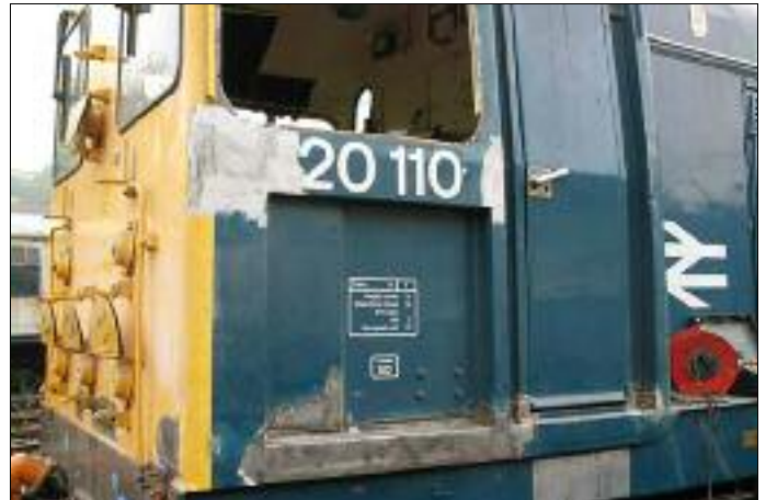
20 110 Driver's side corrosion repairs October 2007. Pete Burrow
