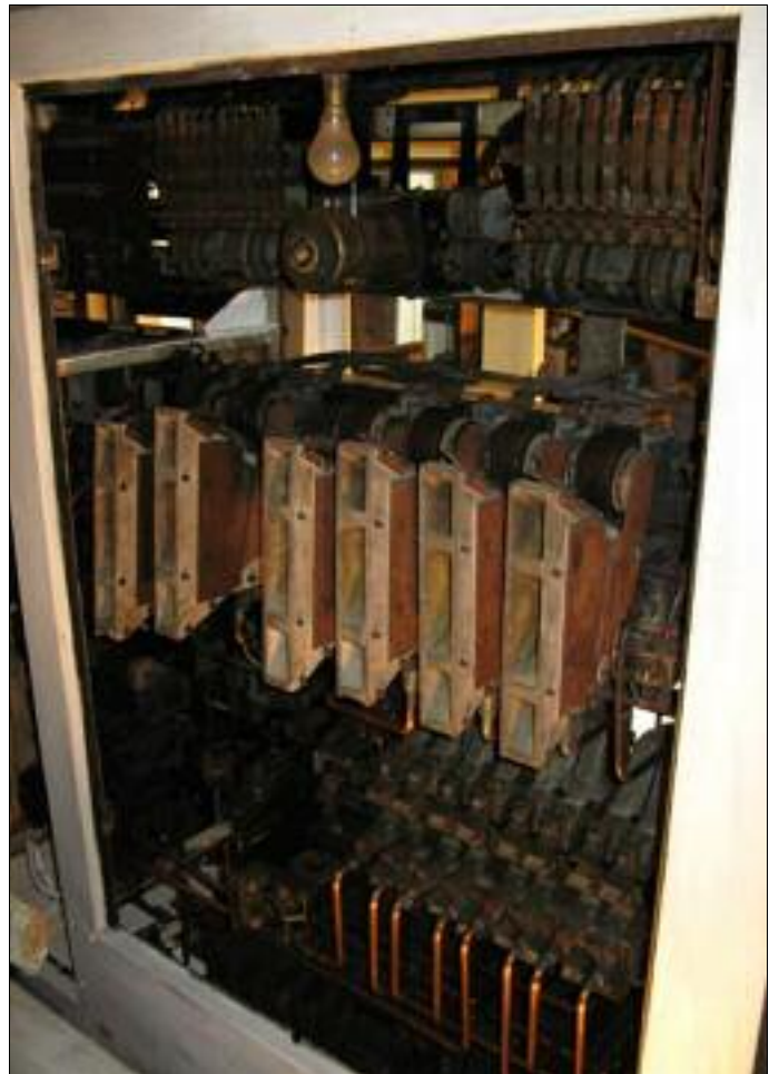
33 002's overhauled and refurbished electrical cubicle after many hours of attention. All missing parts have been sourced.
