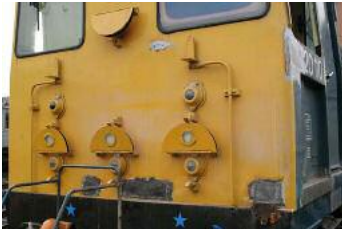
20 110 receiving cab corrosion repairs October 2007. Pete Burrow
