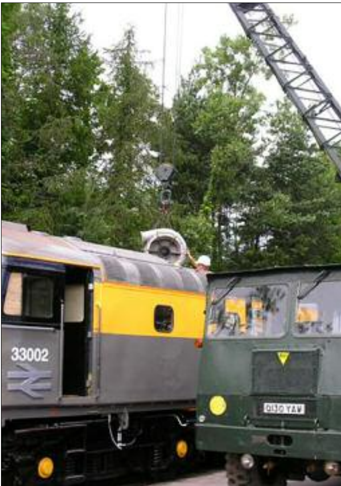
33 002's turbo has been craned out of the loco and dispatched for assessment / overhaul to a company near Barrow Hill Pete Burrow
