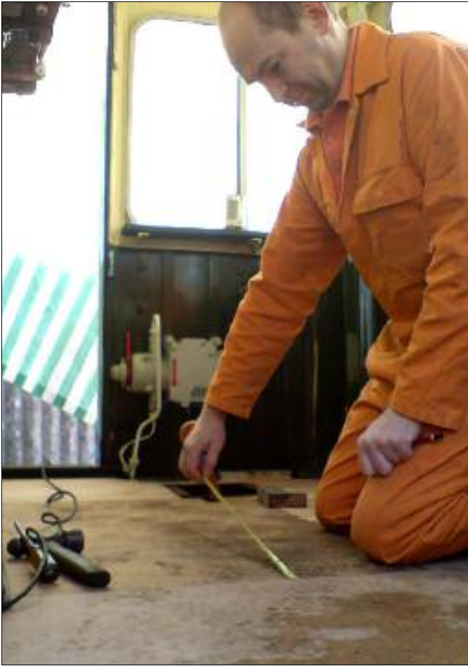
D7612's cab floors have been renewed using plywood covered with brown lino and finished off with brass trim Chris Rees / Phil Seymour
